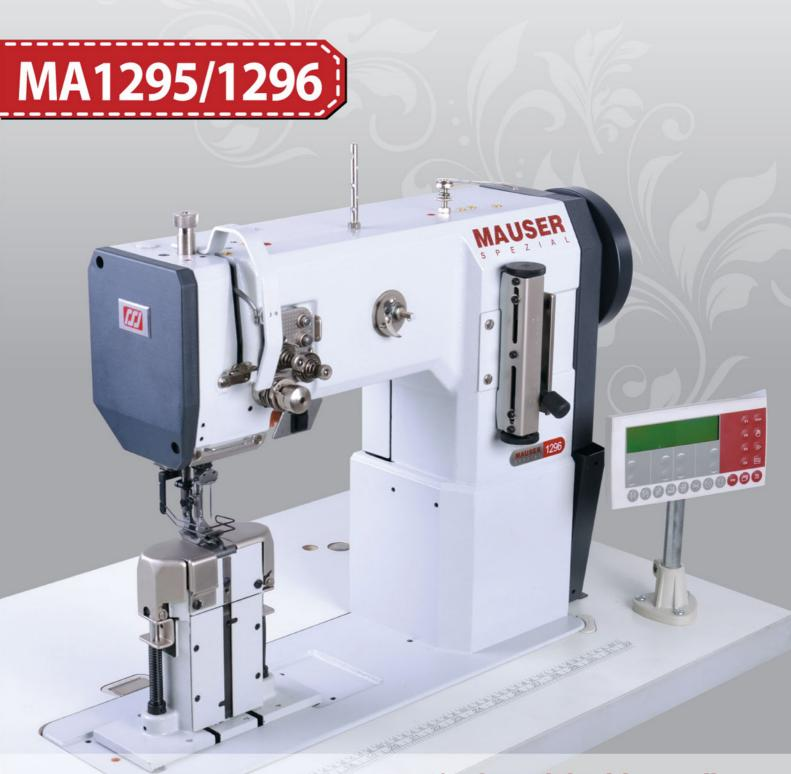
Single and double needle post-bed sewing machine with unison feed
