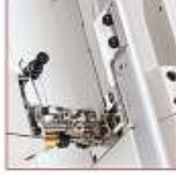
包縫骨壓縫裝置 (倒骨式) Seam Overlock Attachment (Folding Over)
