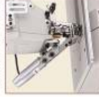
STE: 電動式頂上蓋切線裝置 Electric Top Cover Thread Trimmer
