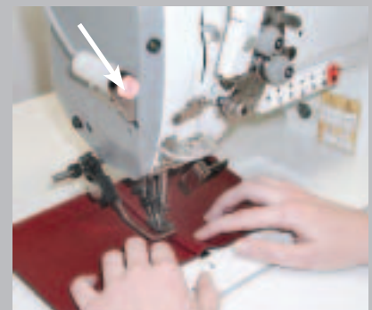
In case of a skipped stitch -> Machine stops automatically -> Signal on -> Start sewing is blocked
