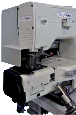
Cylinder arm unit, full lubricate, made by Kansai Japan
